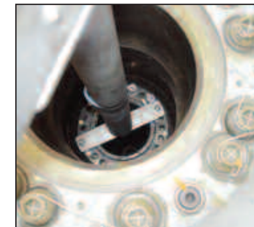
Swench breaking torque on a frozen main rotor mast nut on a UH-60 helicopter using the 750 model, 3/4 inch drive wrench set.
