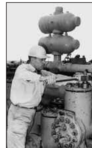
Loosening blowout preventers, christmas tree bolts and nuts on pumps are a cinch for Model #1000 SWENCH. Thin wall box end wrenches are used to reach those "hard to get at" nuts and bolts.
