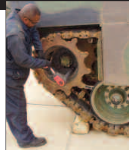
One person breaking torque on the M1 Abrams tank drive sprocket nuts using the 1000 model, 1 inch drive Swench wrench set.
